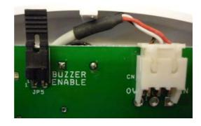
shown and named "BUZZER ENABLE". Hold the tab between your thumb and finger and pull it upwards away from the PCB. The buzzer will no longer sound.
